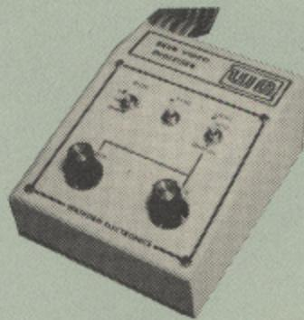
Using any source of composite video (colour or monochrome) and the Watford Beeb Video Digitiser, you can convert an image from your camera into a graphics screen on the BBC Micro.
